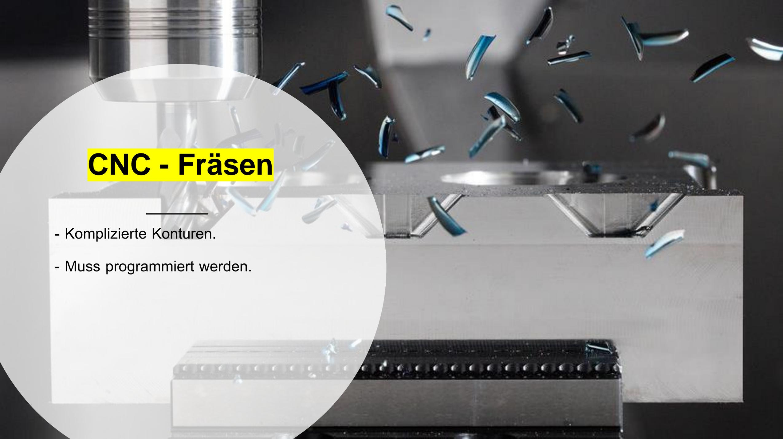
A close-up photograph of a CNC milling operation. A metal cutting tool is positioned above a workpiece, with numerous bright, curved metal shavings being ejected from the cutting zone. The background is dark, highlighting the metallic surfaces and the dynamic nature of the process.
